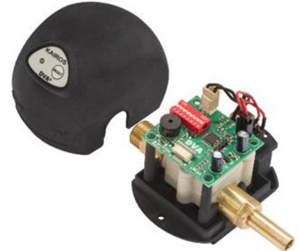
By adjusting the settings on the PCB, **Kairos** can be mounted on multiple cylinder sizes and on all of our models.
